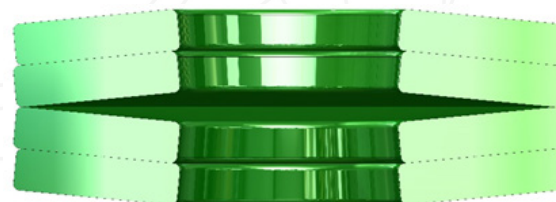
Parallel/Series Doubles load- doubles deflection
